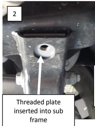
Threaded plate inserted into sub frame
