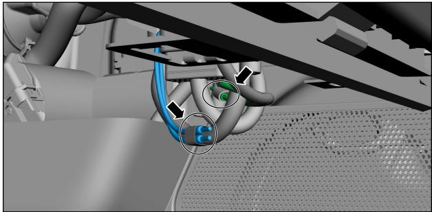
15. Reconnect the battery cable to ground. Torque to 48 lb.in (5.4 Nm).
