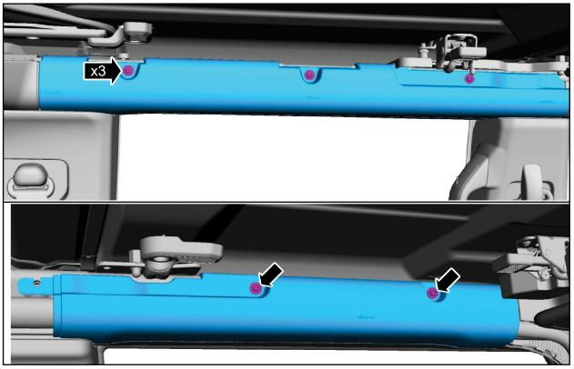
8. Release the clips and the upper tab then slightly position aside the upper A-pillar trim panel for wire routing.
