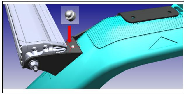
**NOTE:** The roof line brackets should be installed with the light bar mounting slot facing forward and outward.
