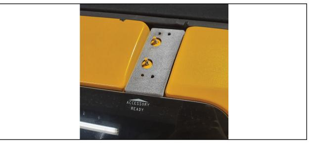
NOTE: The roof line brackets should be installed with the light bar mounting slot facing outward
