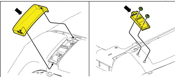
3. Install the top bracket piece to the Rigid roof line bracket using the four small screws.
