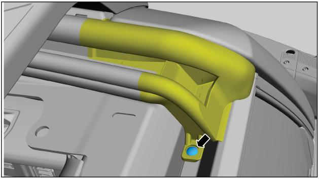
10. Remove the light bar cable insulation tubing carefully up to where the wires enter at the roof line. Route the light bar power and ground wires in between the weather stripping and metal. DO NOT break into the seal or route the wire through the hard top mounting holes. Proper routing is shown below.
