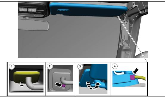
4. Open the fastener cover, remove the fastener and the sun visor clip. Perform this step on both sides.
